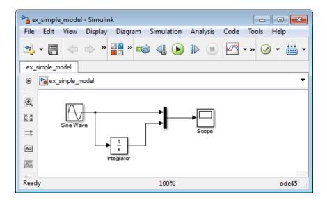
Simulating this model integrates a sine wave signal to a cosine signal and then displays the result, along with the original signal, in a Scope window.
