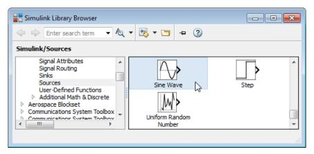
**3** Drag the Sine Wave block to the Simulink Editor. A copy of the Sine Wave block appears in your model.
