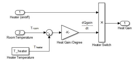
The Inport and Outport blocks create ports that connect this subsystem to other subsystems in your model.
