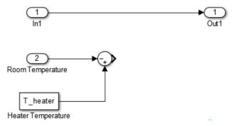
Add labels to the signal lines to help trace model components to the equations and model requirements. Double-click above a signal line and enter a label.
